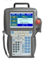
The WeldSaver<sup>™</sup> graphical user interface provides information on device status in real time, with clear visual indicators and descriptions. The interface can be accessed over a network using most JavaScript<sup>™</sup>-enabled web browsers by entering the working IP address of the device.
