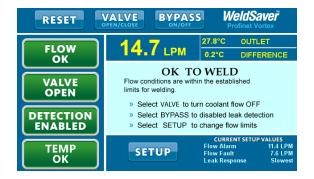
The WeldSaver graphical user interface provides information on device status in real time, with clear visual indicators and descriptions. The interface can be accessed over a network using most JavaScript<sup>™</sup>-enabled web browsers by entering the working IP address of the device.
