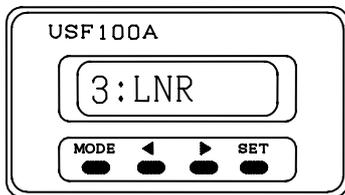
Using **<** and **>** keys, select the setting screen for linearization. When it appeared, press **SET** key.
