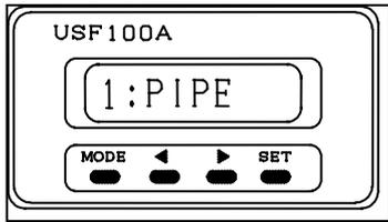
In the condition of the flow indication, press **SET** key while pressing **>** key for over one sec. to display the screen left.
