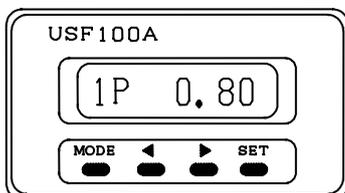
Using **<** and **>** keys, input the indicating flowrate on USF indication which is the lowest compensated value.
