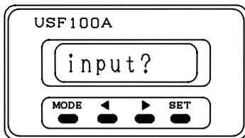
Press **SET** key to move to the input screen of the compensated flowrate.
