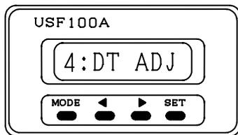
Using **<** and **>** keys, select the setting screen of the compensating value. After it appeared, press **SET** key to proceed to setting screen.
