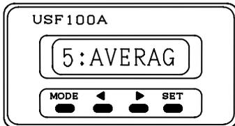
Using and keys input actual flowrates (indicated value at master flowmeter). Press key to store new data and proceed to next step.
