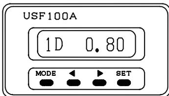
This is the input screen of actual flowrate. Using **<** and **>** keys, input the actual flowrate.
