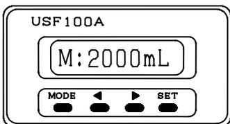
Using **<** and **>** keys, input the instantaneous flow indicating values of the ultrasonic flowmeter. Press **SET** key to stores new data, and to proceed to the next step.
