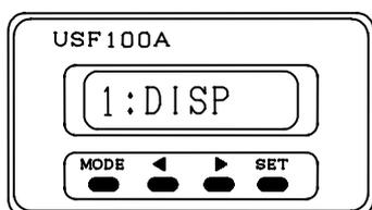
In the flow measurement mode, press **MODE** key to display the screen left.
