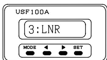
Using  and  keys, select the setting screen for linearization.
