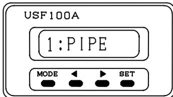
In the condition of the flow indication, press **SET** key while pressing **>** key for over one sec. to display the screen left.
