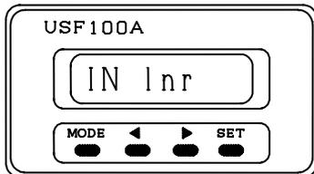
Using **<** and **>** keys, select the input setting screen for compensating flowrates. When it appeared, press **SET** key.
