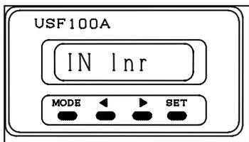
Using **<** and **>** keys, select the input setting screen for compensating flowrates. When it appeared, press **SET** key.
