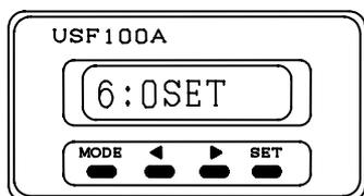
Using **<** and **>** keys, select the screen for zero adjustment.
