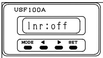
Using **<** and **>** keys, select "lnr : o f f " and press **SET** key.
