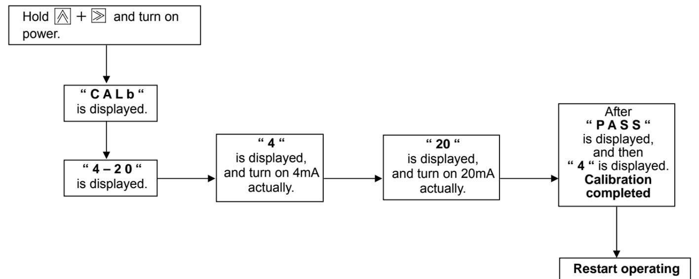
**Note:** Before calibration, check to ensure that the setting of analog input selection (setting of current and voltage input) has been made properly. (For more details, see on page 8.)
