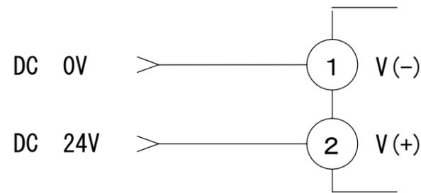
※Install the choke coil (Noise filter) and the like more than 0.29 mH / 1kHz, when wiring. A good result will be appeared, specifically where there may exist an electromagnetic field and noise.
