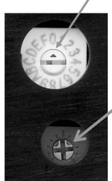
The orientation of the fine adjustment potentiometer is indicated by two indents.
