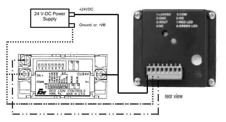
Figure 7: Wiring connections for Digital Display
