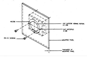
Figure 3: Layout for panel mounting
