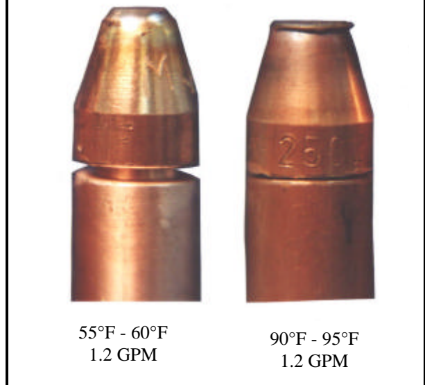
FIGURE 11: EFFECT OF HIGH WATER TEMPERATURE ON CAP REMOVAL
